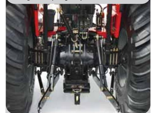
Efficient Ferguson three point linkage
